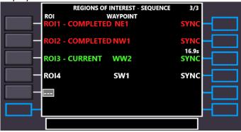
Already passed ROI's are shown in red, the one which is targeted by the current sweep in green and the remaining duration of the sweep in seconds above the green SYNC.
