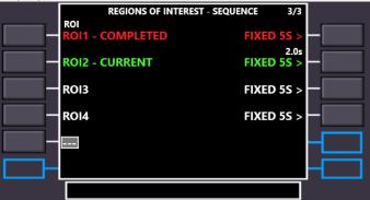
Already passed ROI's are shown in red, the one which is targeted by the current sweep in green and the remaining duration of the sweep in seconds above the green FIXED nS.
