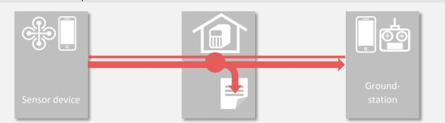
During normal operation the sensor device transmits sensor and location data to the relay server. The data is then fed forward to the groundstation.
