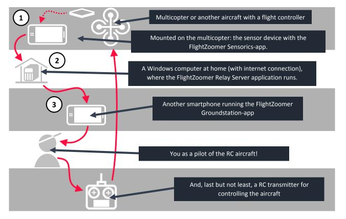
FlightZoomer consists of three components:
