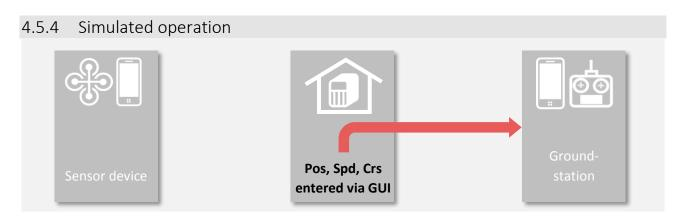
Beside the option to replay logfiles from earlier flights, the flight parameters (location, speed, course and altitude) can also be generated directly by providing these parameters on the relay server GUI. This allows to simulate very precise flight movements again for training purposes and system acquainting.
