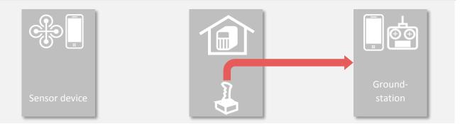
The input for the flight simulation can also come from standard joystick, which is connected to the relay server. This allows to train and inspect the features of the groundstation nearly as realistic as flying with the real model.
